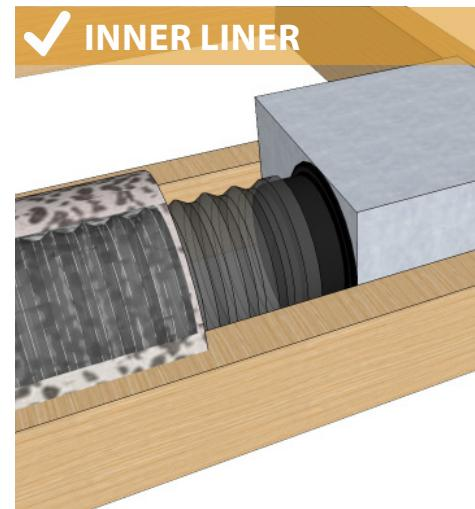
3. After checking the inner liner reaches both the fan collar and the exhaust termination, seal it in place using bucket mastic and zip ties.
