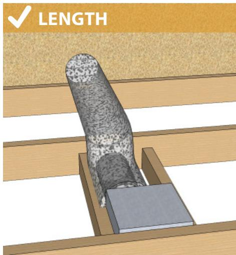
2. Ensure the inner liner is not tucked inside of the insulation or restricting movement of the fan damper.
