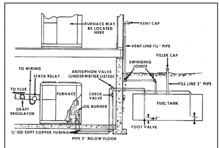
Figure 12.3. Piping Hookup for Buried Outside Tank [4]
