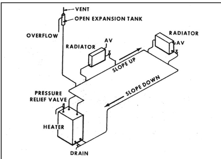
Figure 12.11. One-pipe Gravity Water Heating System [4]
