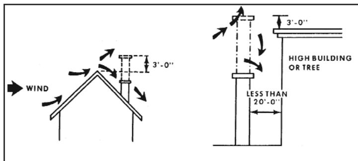
Figure 12.18. Draft Relation to Height of Chimney [4]
