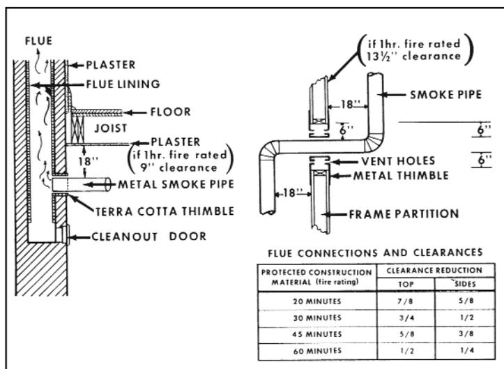
Figure 12.17. Wall and Ceiling Clearance Reduction [4]
