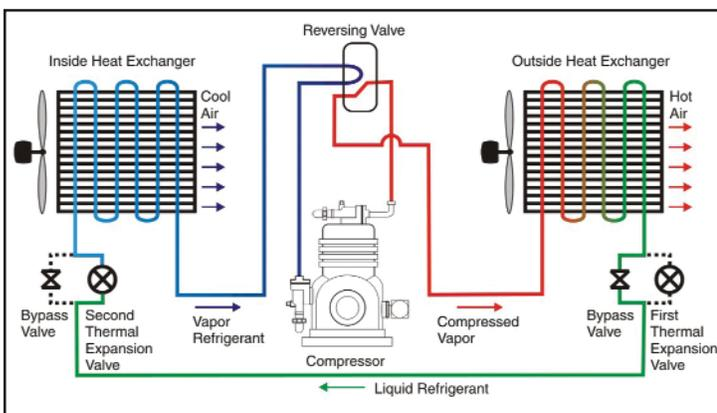
Figure 12.1. Heat Pump in Cooling Mode [2]
