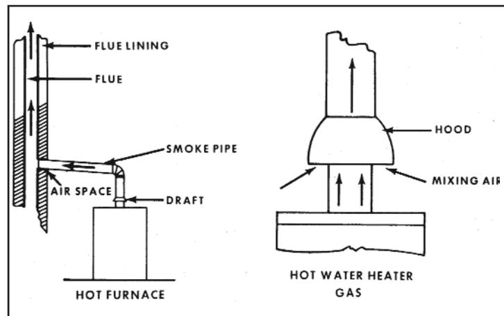
Figure 12.19. Location and Operation of Typical Backdraft Diverter [4]
