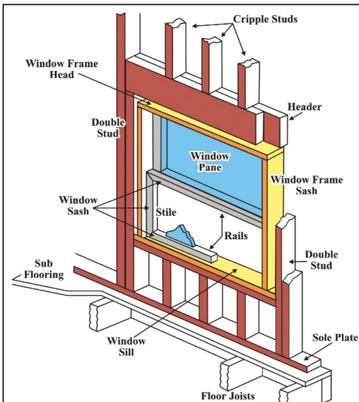
Figure 6.7. Three Dimensional View of a Window [1]
