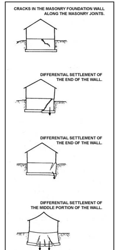
Figure 6.4. Foundation Cracks [4]
